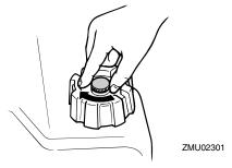
(3) Disconnect the fuel line if you are using an external fuel tank.
